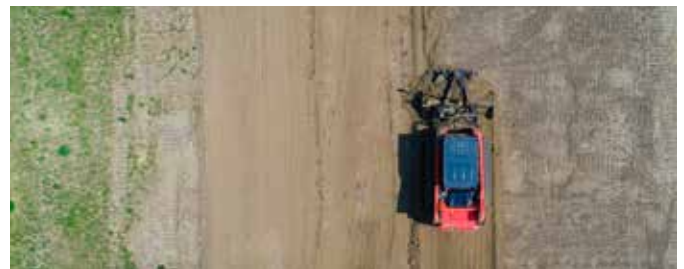
A Kubota SVL97-2 is guided by Topcon's MC Mobile System, applying a 1% fall across a 250-foot-long plot area in Delaware County, Ohio.
