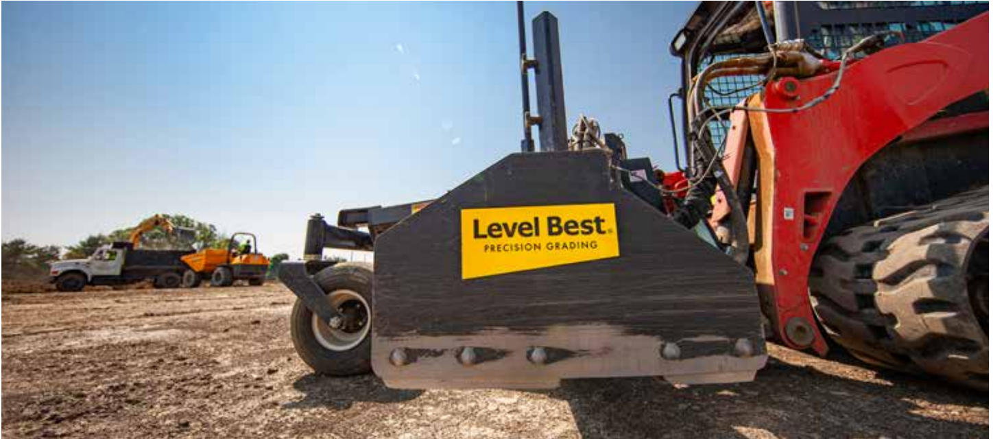
Frye describes the company's four Kubotas as "phenomenal machines." The SVL97-2 has proved a perfect complement to the Level Best grading box, increasing margins on compact grading projects, as well as bike path and baseball diamond installations.
