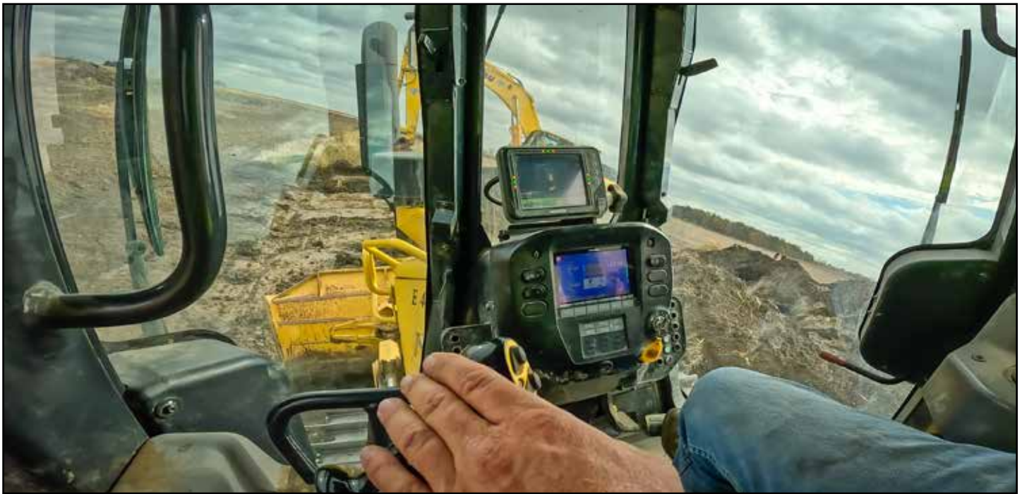
VTF Excavation Operator Jim Moehler at the helm of a Komatsu D51EXi on the Mercer County ditch project. Employing iMC technology, VanTilburg was able to save an entire crew, 50% dozer time, which resulted in 20-30% overall savings on the project. Plus, the mile-long ditch was accurately built, maintaining proper flow to the river outlet.
