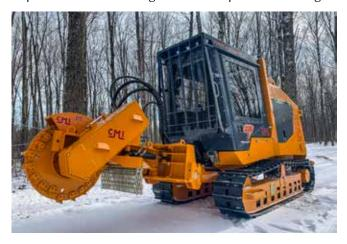
The new S175 will also fit older C175 models since the three-point mount plate is the same. That said, CMI highly recommends contacting your local dealer regarding installation to determine whether in-line, flowcontrol valves are required to slow down the speed of certain functions such as swing cylinders and tilt down.
