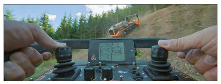
FAE is expanding its RCU series with an exciting, new RCU-75 model. The compact, powerful, remote-controlled tracked carrier is designed to work on hard-to-access areas and steeply-sloping terrain. In fact, the RCU-75 is capable of mulching vegetation up to 6" in diameter while climbing slopes up to 55 degrees.
