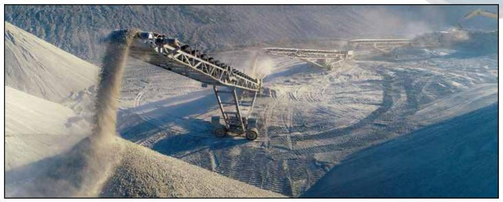
Robert Jacobs Incorporated's Astec GT440 Mobile HSI Crusher Plant relentlessly stockpiles crushed shale into 3,000-ton cones. Along with larger aggregate, liners and rubber chips, the finely-crushed shale is used as an effective surrogate for clay to line a large, new landfill cell.
