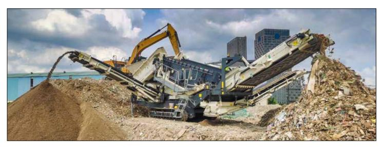
Terex Ecotec's TRS 550 Recycling Screen is a highly efficient and versatile mobile screening machine, with a specialist screenbox from Spaleck, the industry-leading German manufacturer. The proven Terex platform lends itself to superior, screening performance particularly in the more challenging, wet and sticky conditions that typify early-season production in the mulch industry, for example.
