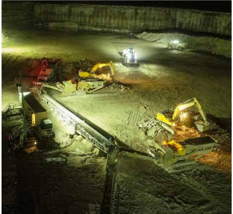
The main crusher—a 3862 track jaw crusher—had a bearing failure this summer. The company needed a fill-in replacement while the machine was being repaired, and Columbus Equipment Company was able to supply two machines—an FT4250 horizontal impact crusher and an FT2650 jaw crusher—both tracked, portable machines.
